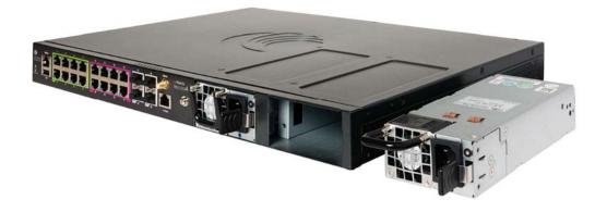
Ensure that the CRPS is installed in the correct orientation. The handle will be located on the left, while the latching tab will be located on the right side of the CRPS.
