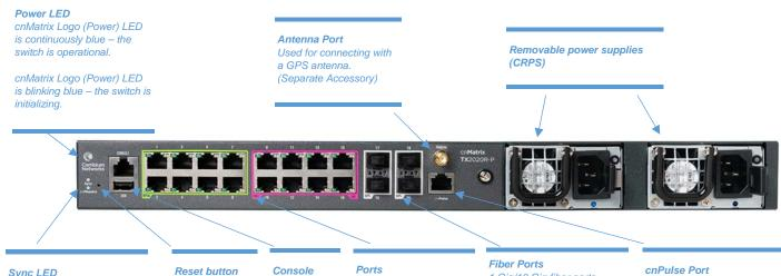
Sync LED Satellite lock from antenna or cnPulse: Green No satellite lock: Amber
