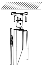
Figure 2-2 Install the Camera to the Ceiling
