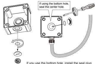
If you use the bottom hole, install the seal plug to the unused hole in the center.
