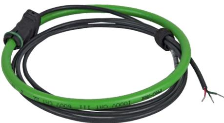
Rogowski coils are slightly less accurate than Split-Core CTs but offer an even larger current range up to 50,000 Amps. The PQ Edge supports Rogowski coils without the need for an integrator, they can be connected directly to the current terminals.
