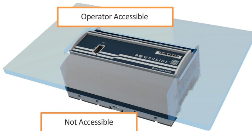
The operator must be protected from the hazardous screw terminal blocks by a barrier. The screw terminal blocks must be made “not accessible,” as defined in UL /IEC 61010-1 6.2, using an enclosure or barrier that meets the rigidity requirements of UL /IEC 61010-1 8.1 and that requires a tool to remove.
