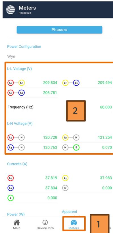
2. Check the current readings, if you see that your current readings are negative and you are not generating power, then the CT may be installed backwards, or it may be wired backwards. See [Connecting the Current Sensors](#) for wiring instructions and see [Fix connection errors](#) to fix this in the configuration of the device without the need to rewire / reinstall the CTs. You will also need to set CT ratios, see [Configuration: AC Currents](#) for more details.
