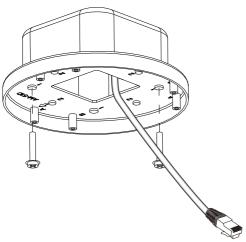
3. Remove dome cover of camera and fasten camera to adapter plate.
