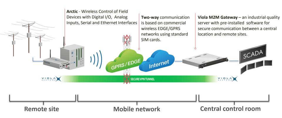
**Operator independent Viola M2M Solution** - the IP address does not need to be fixed, also dynamic IP addresses works. Always in Viola M2M solution, the M2M gateway provides a fixed IP address for all remote devices. Consequently, all of the remote devices have always a fixed IP address even if the address provided by the mobile operator is dynamic
