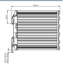
Dimension  $134 \times 100 \times 122 \text{ mm} (5.25 \times 3.93 \times 4.80 \text{ in})$
