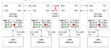
If an optical fibre segment fails, all communication with units beyond the faulty fibre segment will be lost. To determine which fibre segment has failed, look at the FL L, CH 1 and CH 2 LEDs as show in the picture above.
