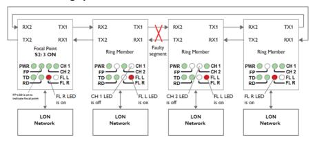
If an optical fibre segment fails, the LRW-702-F2 unit configured as focal point will reconfigure the system so that data is sent and received over the otherwise redundant fibre pair.
